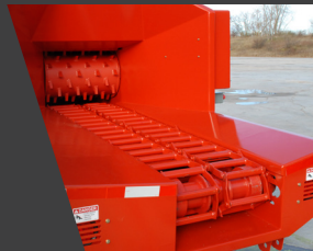
A 6' (1.83 m) infeed bed with live WDH-110 chain drive
