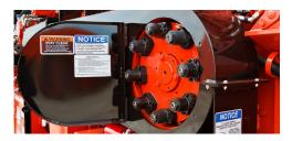
Externally adjustable break-away torque limiter protects the driveline and hammermill from catastrophic damage.
