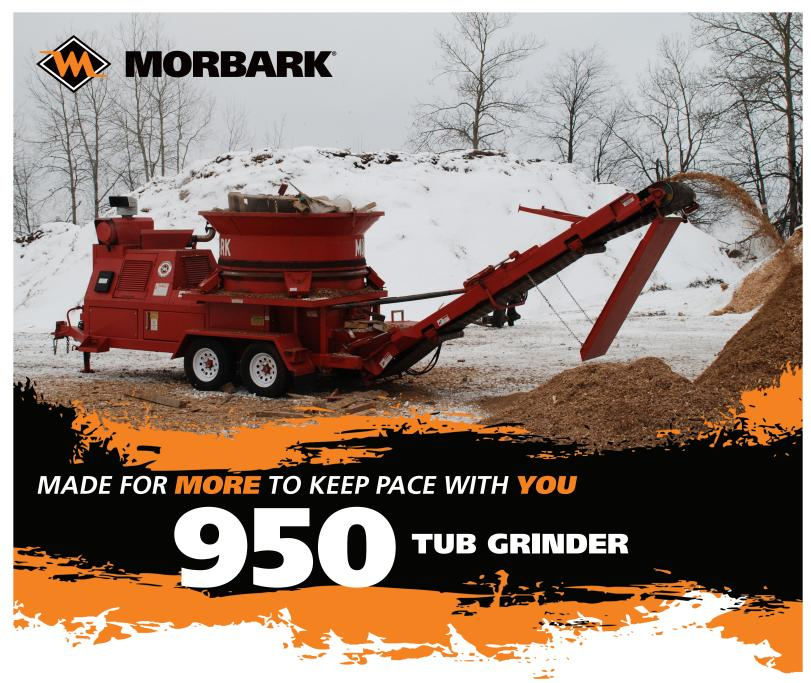
Compact and easy-to-haul, the **Morbark 950 Tub Grinder** is ideal for converting yard and wood waste, pallets and other mixed woody feedstocks into saleable products. The 950 tub grinder is equipped with a proven drive line protection system that protects against catastrophic damage from contaminants.
