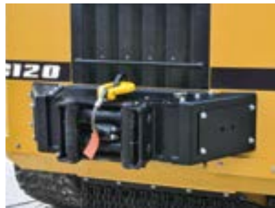
Hydraulic rear winch with 12,000-pound capacity.
