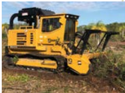
102 gpm cutter system provides hydraulic power to 7-foot Predator mulcher head.
