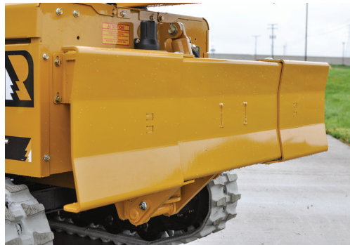
The wide hydraulic backfill blade saves time during clean up and can easily be folded in for passing through gates.
