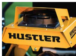
9" fan & high capacity oil cooler with hot oil shuttle
