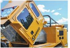
Hydraulic cab tilt for complete access to service components.
