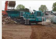
Tracks **Power Unit Bypass Conveyor (option)** Width: 400mm (15.7") Width: 500mm (20") Tier 3/Stage 3A: CAT 7.1 Tier 3 ACERT, 186kW (250hp) Discharge height: 2.03m (6'8") Tier 4F/Stage 4: CAT C7.1 205kW (280hp)
