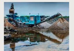
Feeder Crusher Wear resistant feed hopper Vibrating pan and grizzly feeder Twin apron, 4 bar impact crusher Length: 4.87m (15'12") Length: 4.3m (14'1") Feed Opening: 1370mm x 911mm (54" x 36") Width: 2.62m (8'7") Width: 1.26m (4'2") Min. CSS: 75mm (3")\* upper apron Min. CSS: 35mm (1.4") lower apron Capacity: 7m3 (9.2yds3) Grizzly length: 2m (6' 6") Power Unit Tier 3/Stage 3A:
