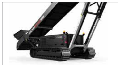
With 400mm dual speed tracks as standard the AggreStac offers speed and control during installation across any terrain
