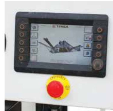
Local machine control panel
